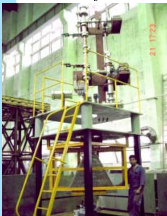
Trial assembly of 10 MeV, 10 kW RF Electron Linac
