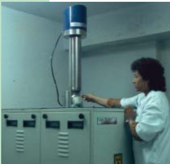
Tissue grafts being irradiated in the Gamma Chamber-1200 in the TMH Tissue Bank. The equipment has been manufactured by BRIT.
