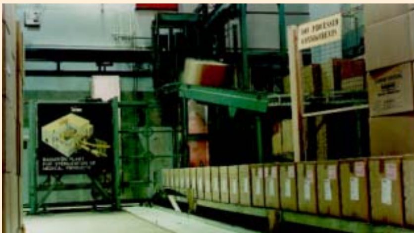
Medical products sterilized by gamma rays (top) and Isomed plant at Trombay that offers sterilization services to medical industry
