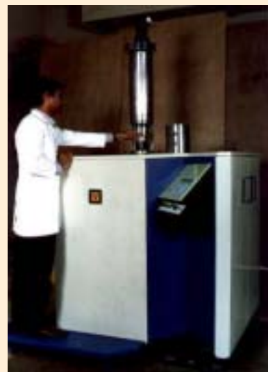
Gamma chamber irradiator developed by BRIT
