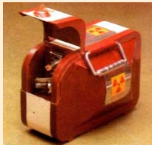
Roli camera for radiography. The camera is being marketed by BRIT
