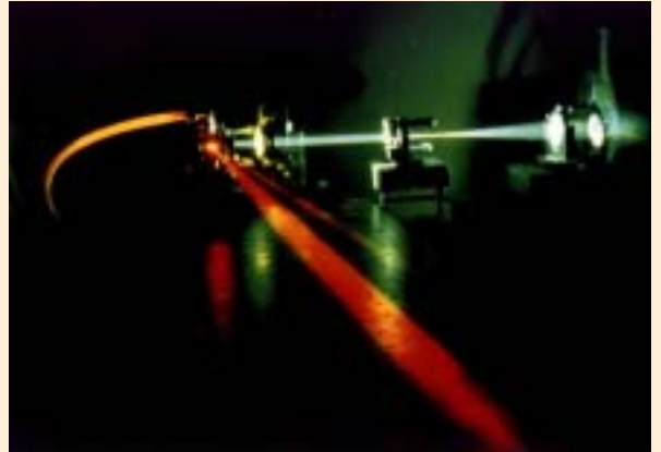
Dye laser pumped Copper Vapour Laser. These lasers have been developed at the Centre for Advanced Technology, Indore, Madhya Pradesh
